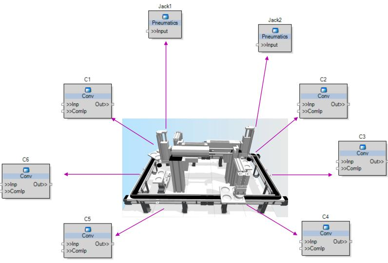
Each function block type implements basic control services for the mechatronic component.
