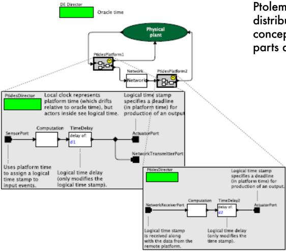
Ptolemy and pTides is a semantic framework for distributed CPS that uses a uniform time concept for both physical and computational parts developed at UCLA Berkeley.
